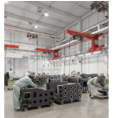
The right angles of each spindle housing are hand-scraped to the highest precision.
